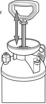
To **lock** the handle (from the unlocked position), make sure it is pushed all the way down to the tank and gently **turn it counterclockwise** until you feel a "click".
