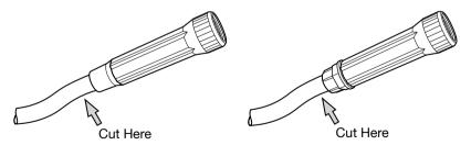
Cut the hose to start installing the new plastic handle assemble.
