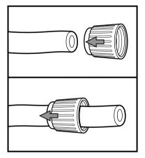
Step-3: Push the plastic insert into the hose; press it on the table until it is flush.
