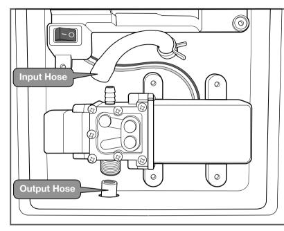
After the Charging Dock and the Pump Module are placed into the chamber, connect the hoses.
