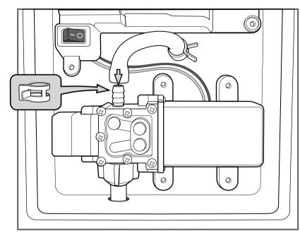
Connect the Input Hose to the input pipe of the new Pump Module and secure it using the hose clamp from the previous pump.
