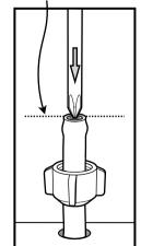
4) Insert the hose into the output pipe of the pump: push until it stops going further.
